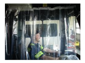
While their plexiglass shield is on order, their interim barrier is a plastic curtain that goes from ceiling to floor. Drivers are directed to have the curtain closed during the boarding process, and to pull the curtain back so they can clearly see their right-hand mirror once the bus is in motion. Maintenance staff installed the cable at the top first.
